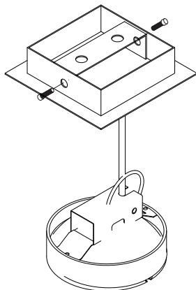
3 Align the lamp rosette with the side holes of the support and start.
