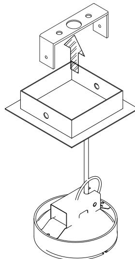
1 Drill the wall where you going to place the lamp. Insert in the wall the plugs suitable for it. Screw the ceiling support to the wall.
