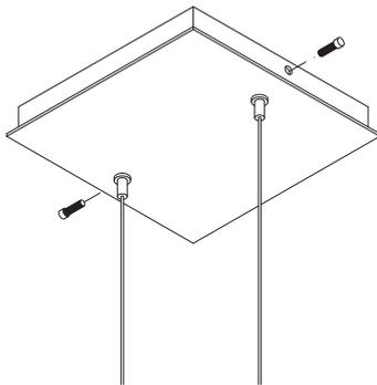
**3** Align the lamp rosette with the side holes of the support and start.
