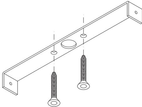
**1** Drill the wall where you going to place the lamp. Insert in the wall the plugs suitable for it. Screw the ceiling support to the wall.
