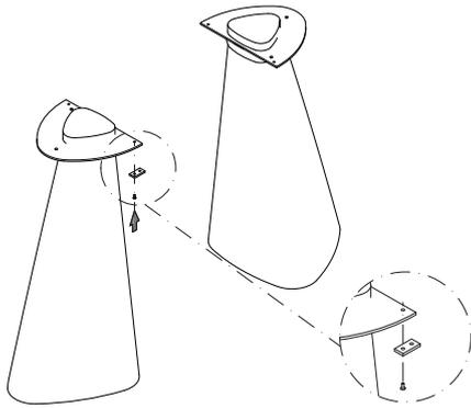
**1** Screw the small metal plates (2 pcs.) to the main plate of the leg.
