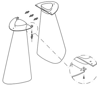
**2** Block the 2 legs. Screw the two small metal plates.
