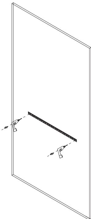
1 Screw the bracket to the panel.
