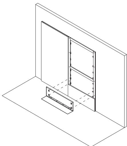
3 Hook the panel with the shelf through the pre-installed frame supports and the corresponding ones pre-installed on the panel. Repeat the operations nr. 2 - 3 for all the panels with the shelves to be installed.
