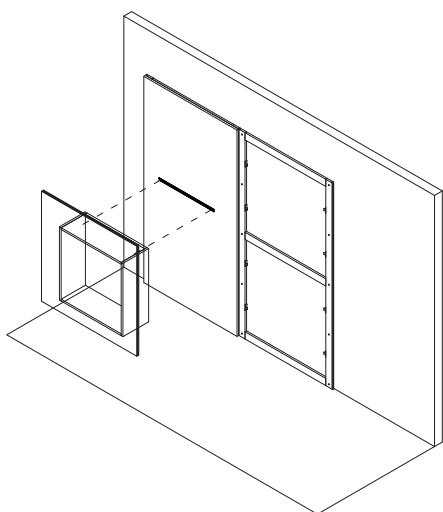
3 Hook the hanging unit through the pre-installed supports.
