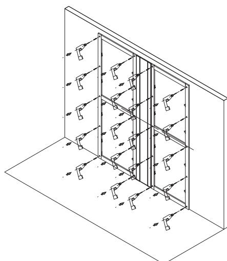
**4** Drill the frames and the wall. Insert in the wall the plugs suitable for the existent wall. Then screw the frames.
