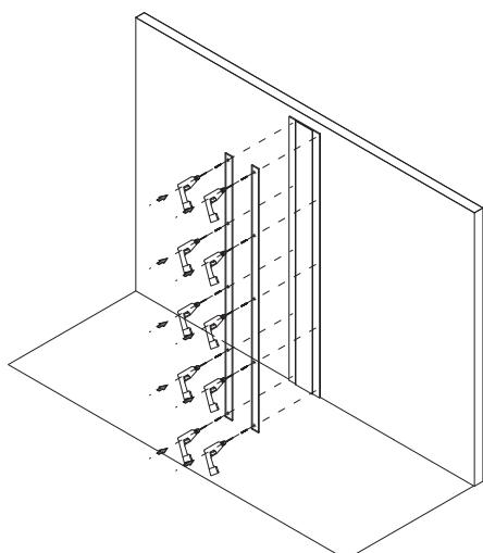
**3** Screw the structure to the panel.
