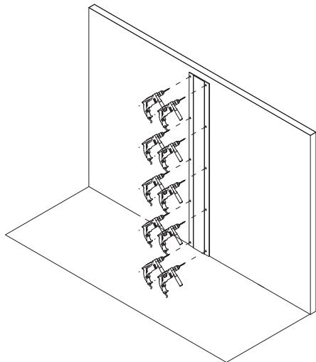
**1** Drill the panel with the marble and the wall. Insert in the wall the plugs suitable for the existent wall.
