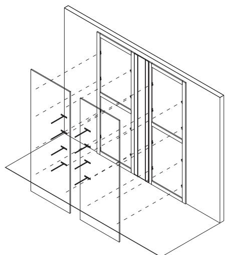
7 Hook the wall panels with the shelf support through the pre-installed frame supports and the corresponding ones pre-installed on the panel.
