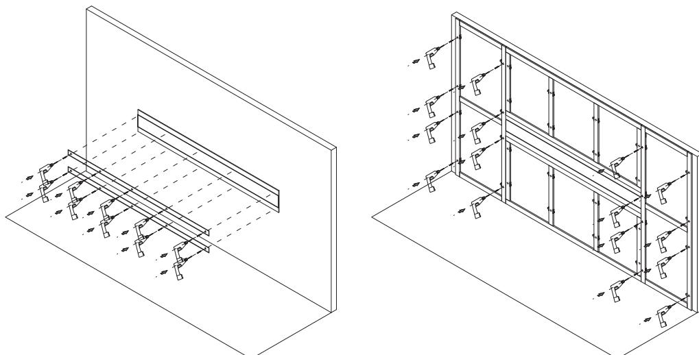
**3** Screw the structure to the panel.
