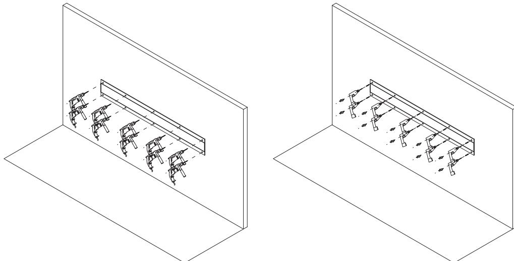
**1** Drill the panel with the marble and the wall. Insert in the wall the plugs suitable for the existent wall.
