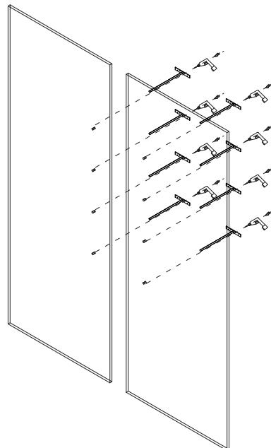
6 Screw the retractable shelf support to the panel.
